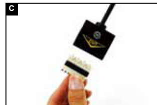
4-pair impact tool seats connecting blocks.
