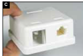
Align the jack to the slot .
