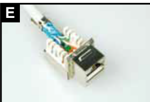
E Put the cap into keystone jack according to the color code.
