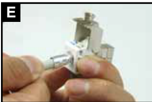
Put the cap into keystone jack according to the color code.
