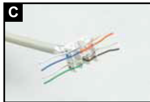
Insert each wire into the appropriate channel according to the color code on the module.
