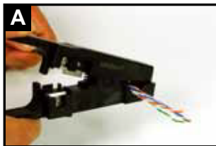
Strip approximate 4cm of the cable jacket.
