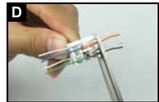
Cut the surplus wires.
