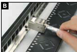
Position the shielded keystone jack for installation.
